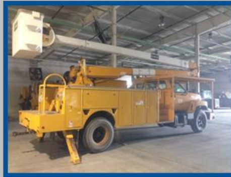
Bucket Truck Lift 52' Height Range
