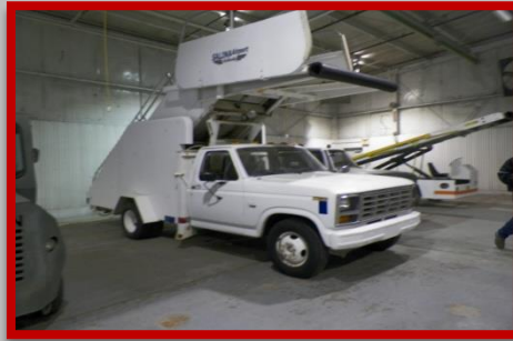
PS1: F350 Self-Propelled Passenger Air Stair See next page for height range
