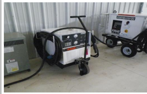
Hobart AC Ground Power Unit 28 VDC Solid State 3ph/208-230-460V/60Hz
