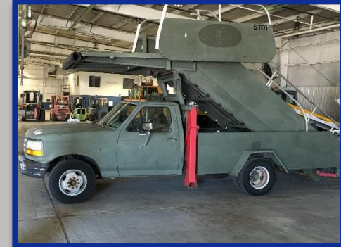
PS4: Self Propelled Passenger Air Stair See next page for height range
