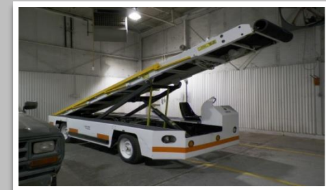
S&S Tug Mobile Belt Loader 11' Height Range
